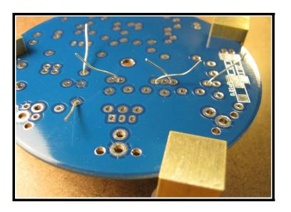
With a BRASS SET in place, the board will now be raised high enough to clear any parts installed on the board thereby providing a perfectly stable platform for soldering the components.
